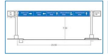
**2. Gantry Advertisements**: These are advertisements affixed to a large frame like overhead structure on the road and supported at two opposite ends of the road ends with pillars. It is used to display signages to vehicles on roads.
