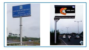
**3. Unipole**: It is type of hoarding with a single pole like support, hence the name Unipole. It could be in conventional format such as billboard with poster or its digital version with LED display screen.
